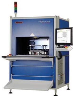
Leister: Dynamic Mask prototype for high-flexible simultaneous laser welding + schematic (fiber laser 1070nm)
