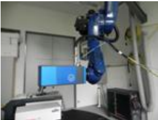
Figure 1: ARGES' "Elephant" F-theta-less scanner, mounted at roboter arm. Laser radiation enters scanner via QBH connector, internally mounted fixed collimating lens and shiftable focussing lens
