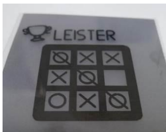
Figure 2: Sample showing simultaneous welding (cup) and contour welding (matrice) with different spot sizes realized within a single scanner run
