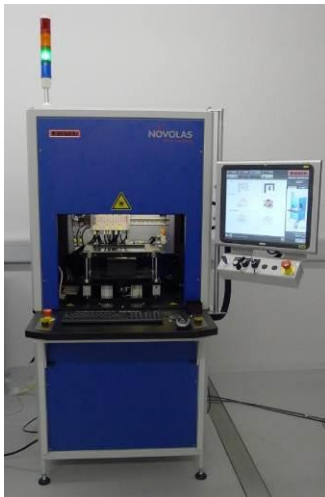
Figure 1: Prototype machine featuring a highly variable LCoS beam shaping system
