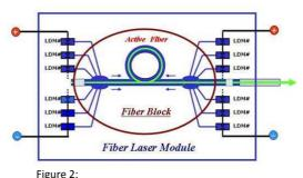
Typical layout for a diode pumped fiber laser
