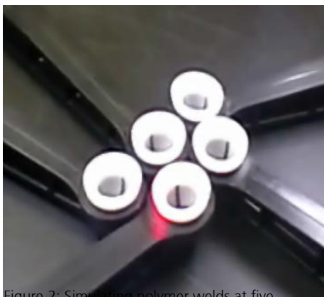
Figure 2: Simulating polymer welds at five arbitrarily arranged white rings with a red laser pointer.
