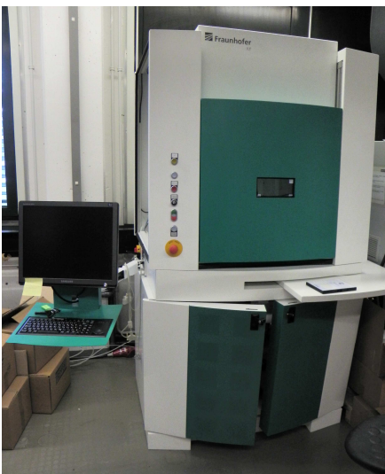
Figure 2: Welding facility including ARGES-Scanner, IPG 1,5 \mu m fiber laser and antenna adapted clamping.
